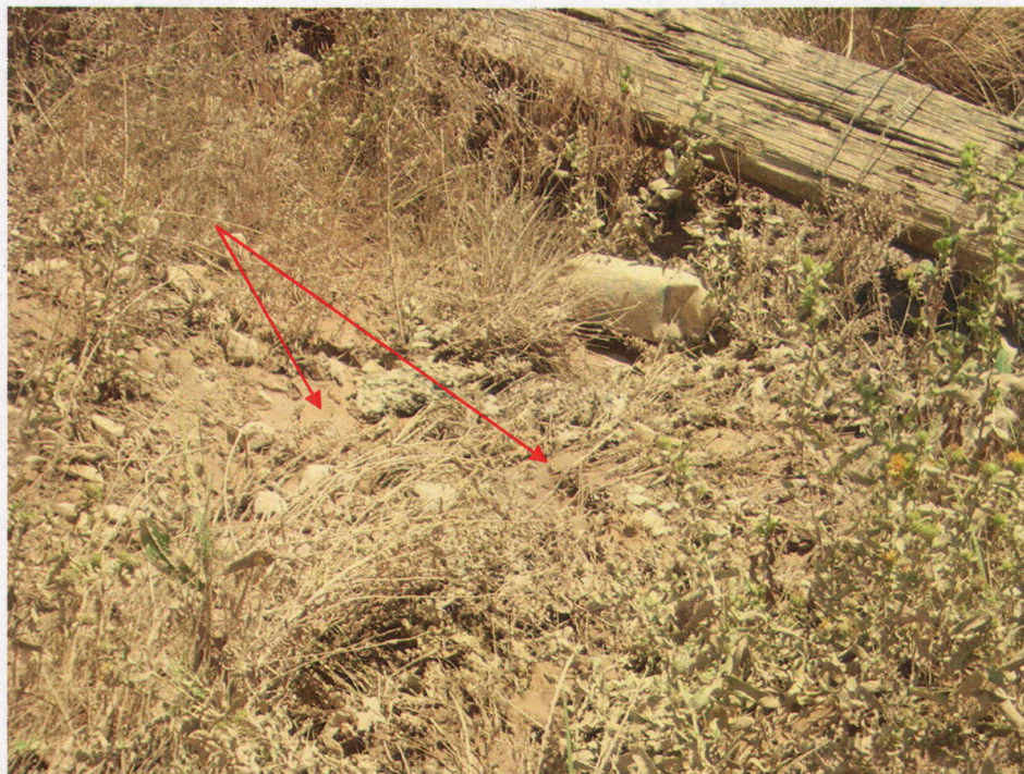
Photo No. 12 – Pictured is the approximate location of the outlet to the County constructed culvert. Photo was taken to again document the condition of existing grasses and other vegetation located along the spill pathway. Note the deposition of dump material (coffee color when wet), red arrows.
